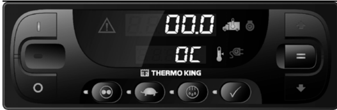
Figure 6: Standard HMI Control Panel
